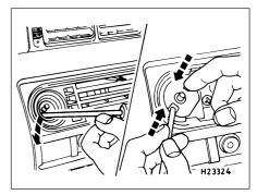
4.23 Heater fan motor control switch removal
